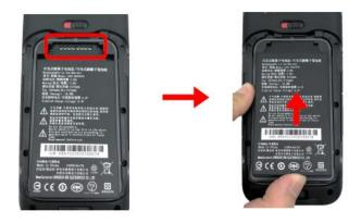
4. Press down the battery to secure in place.
